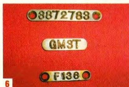
6 A set of casting number, pattern number, and casting date brass tags from the Saginaw Foundry. The characters were individually soldered to the tags
