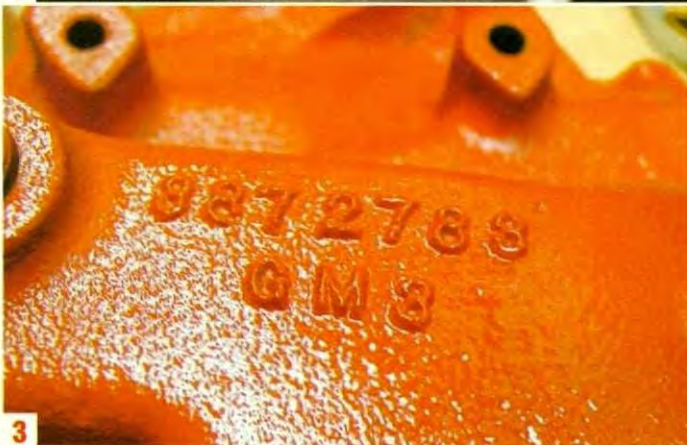
1 A typical casting number on a cylinder head, along with its date. E 23 7 denotes May 23, 1967.
