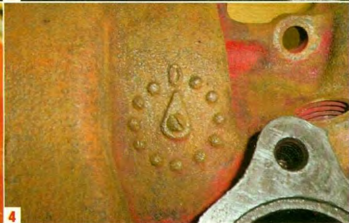
3 The "GM3" pattern number is visible below the casting number on this intake manifold; many identical patterns were required for high-volume castings, and each was numbered.
