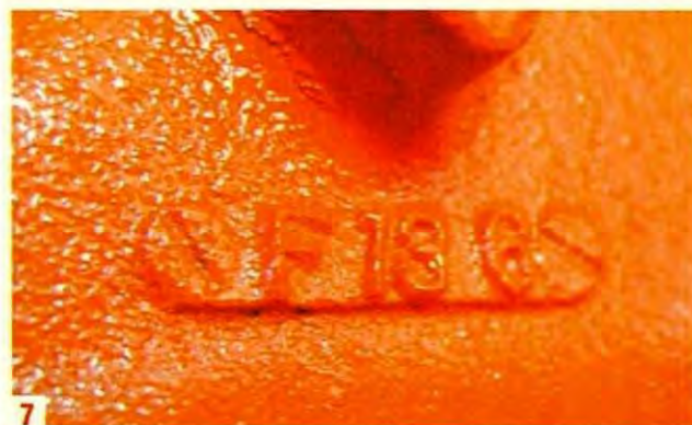
7 The June 13, 1966 casting date that started my research project on the 3872783 intake manifold.
