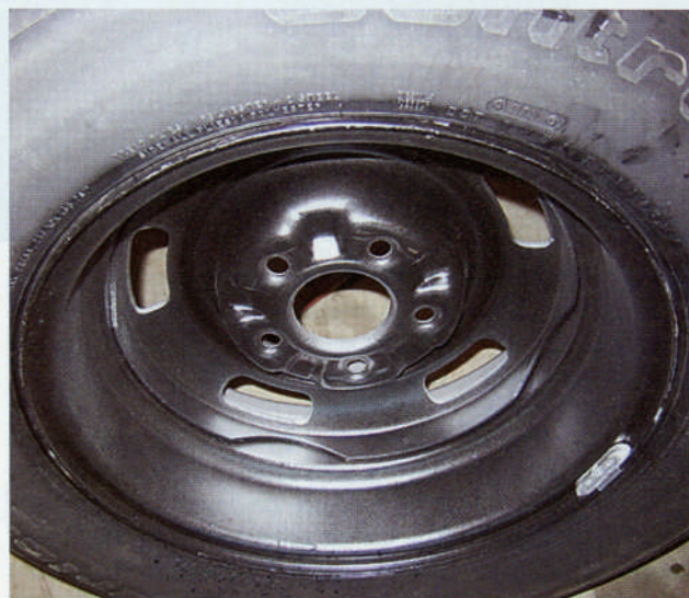
The back side of a factory rally wheel, showing the semi-gloss black primer and faint shadows of argent silver overspray through the slots from the front side.
