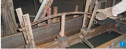
For C1s, steelmakers no longer produce the grooved raw material originally used, so C1 owners should focus on having their original springs re-arched. For C2/C3s, the SAE 5160 alloy steel (premium leaf spring steel used by Eaton for ALL of their springs) is no longer produced in the original .214" and .194" thicknesses, so the next-closest thicknesses are used, with the spring camber adjusted to maintain original ride height.
